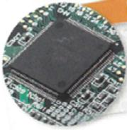
A **microcontroller** is a type of IC that is programmed to perform specific tasks in a wide variety of electronic devices. It contains memory, programmable input/output peripherals and a processor all on one chip – it is essentially a tiny computer.
