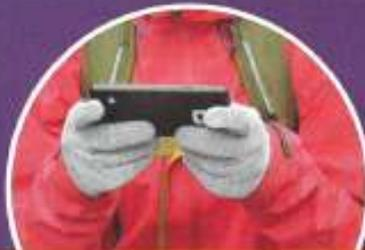
**Conductive textiles** conduct electricity. Metal fibres are either spun into the fabric or metal-based powders are impregnated into the fabric.
