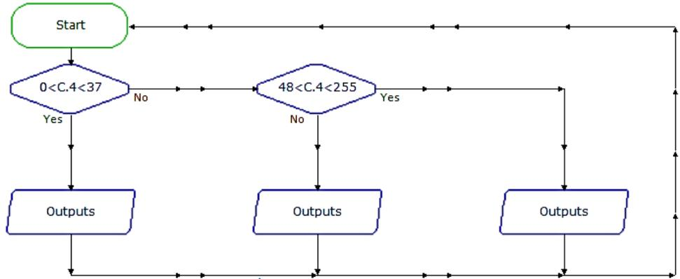
Each output is connected to a different coloured LED. By turning 'on' one output and turning 'off' the other two, it will change the LED depending on the number coming from the Thermistor on C4.
