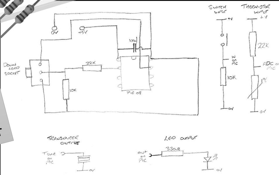
Design an electronic circuit for a bedroom burglar alarm using the PIC microcontroller circuit above as a starting point:
