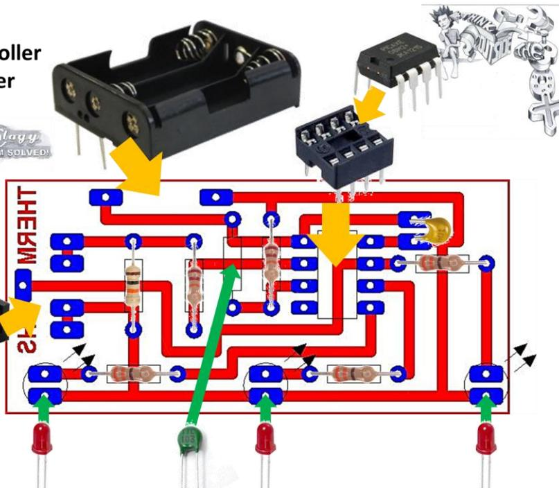
Use a paperclip to set the height of the LED and Thermistor on the reverse side of the board.
