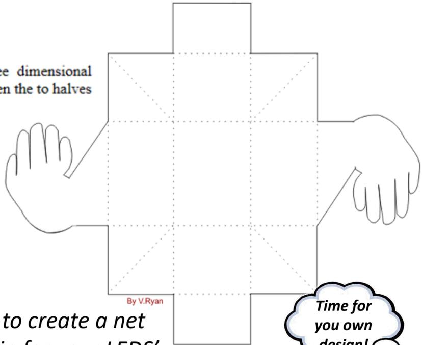
Use layout sheets provided to create a net with the appropriate holes in for your LEDs' and thermistor to show through.
