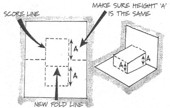
This is the same principle as the previous incised mechanism - only the fold line has moved to create a different shape.
