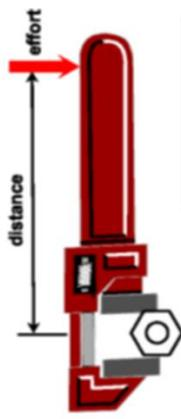
$$\text{Torque} = \text{Effort (newtons)} \times \text{Distance (metres)}$$
