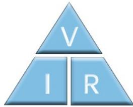
$$\text{Resistance (R)} = \frac{\text{Voltage (V)}}{\text{Current (I)}}$$
