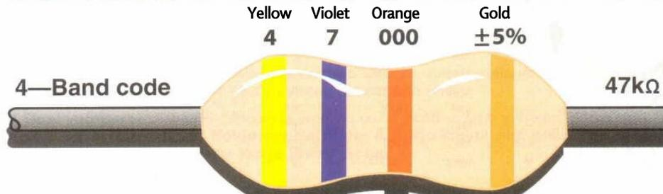
The function of a resistor is to oppose the flow of current in a circuit.
