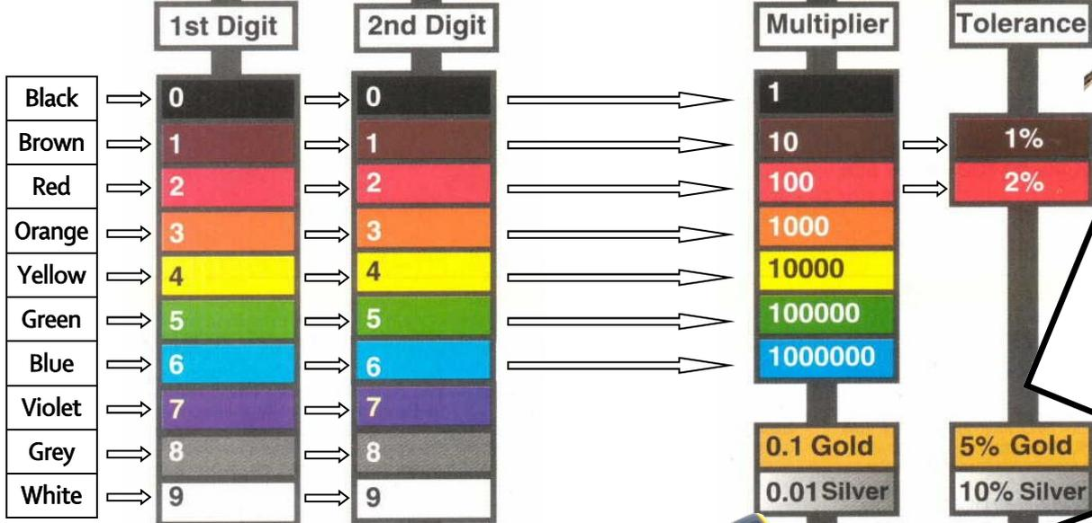
Resistors have different values of resistance to the flow of current.
