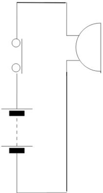
The aim is to move the handle around the wire shape without touching it. If the handle touches the wire a buzzer sounds. A basic circuit for this is a battery, buzzer and switch using crimp connectors to make the joints. This is shown below on the left. A more complex version of this could use a Thyristor to latch the sound on when touched. We can model this on Crocodile Technology later in the project and would use a PCB to make it. The circuit for this is shown on the right.
