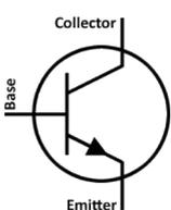
Transistors are like electronic switches. They turn on and off depending on the voltage that is connected to the 'Base' leg. This then allows current to flow through from the 'collector' to the 'emitter'.
