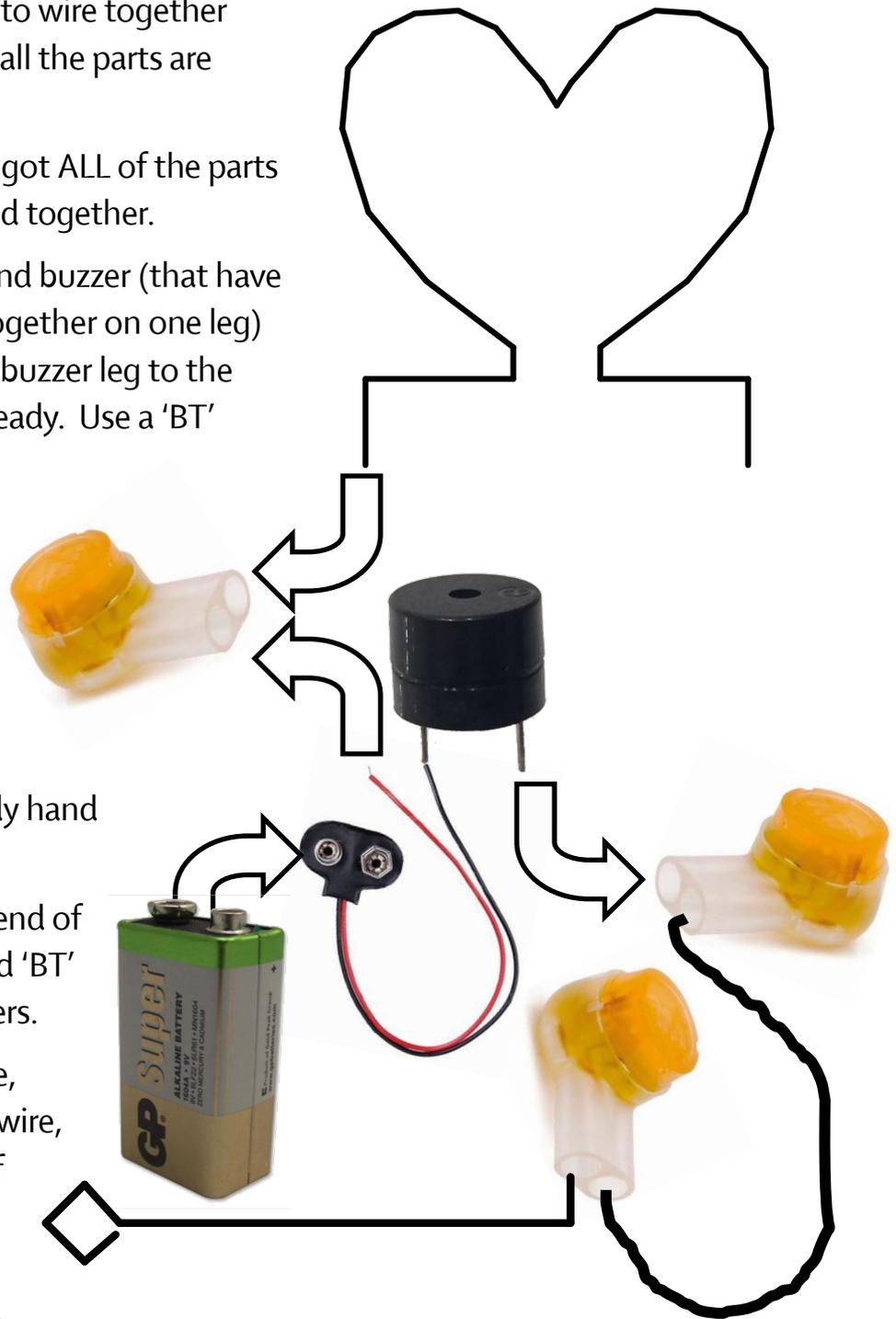
5. Attach the free wire from the battery snap connector to one end of the shaped wire inside your case using a 3rd 'BT' crimp connector. This is the tricky part!
