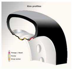
A section of a tyre on a well based one piece rim. When removing or refitting a tyre the bead is pushed into the well allowing the tyre to be levered over the rim.
