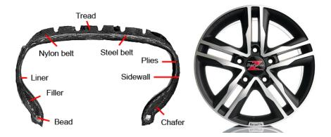
Refitting tyres Before refitting a tyre, the sidewall, bead and inside case of the tyre should be carefully examined for damage. The bead is then lubricated with a special tyre soap or bead lubricant to help it slide over the rim easily and without damage.
